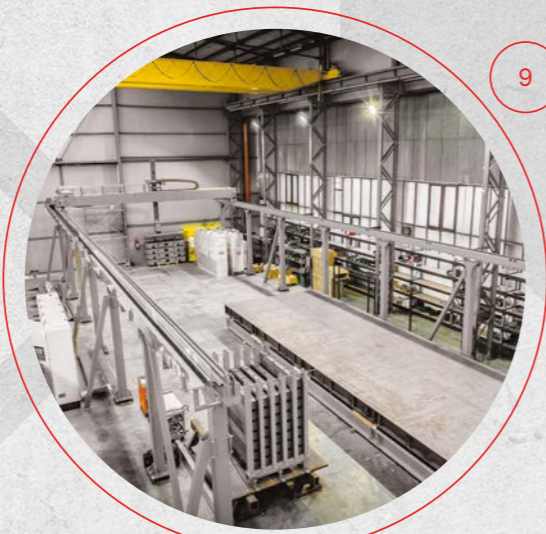
Demoulding area for the magnetic casting separators
